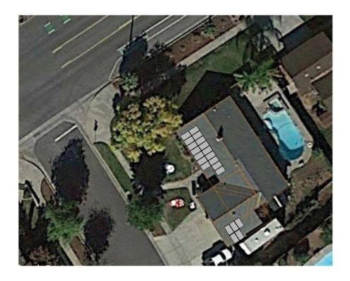
current current recommends a 6kW Roof Mounted Solar system.
